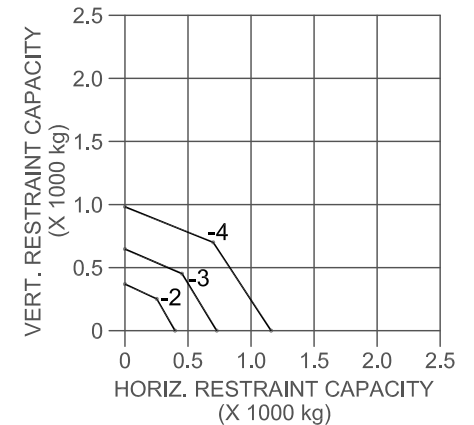
ATTACHED TO CONCRETE WITH KAABS ANCHOR
