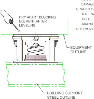
6) DO NOT ATTEMPT TO MOVE ISOLATORS LATERALLY WITH THE WEIGHT OF THE EQUIPMENT ON THEM. IF IT IS NECESSARY TO MOVE THE EQUIPMENT, REMOVE THE EQUIPMENT FROM THE ISOLATORS FIRST. FAILURE TO FOLLOW THIS PROCEDURE COULD RESULT IN DAMAGE TO THE ISOLATORS
