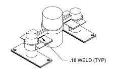
However, if the pipe is expected to grow more than it shrinks (or vice versa), it can be offset to allow the full range of growth/shrinkage to be accommodated over the active travel range of the guide.
