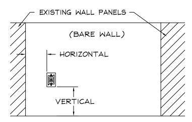
MEASURE LOCATION OF EXTENSION ON THE WALL AND TRANSFER THESE DIMENSIONS TO THE BACK OF THE WALL PANEL
