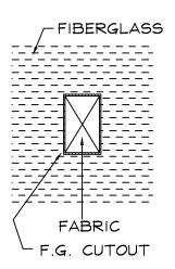
CUT "X" IN FABRIC, SPRAY FABRIC WITH ADHESIVE. PULL FABRIC THROUGH AND ADHERE TO BACK OF PANEL
