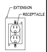
INSTALL OUTLET EXTENSION TO WALL OUTLET PER MANUFACTURER'S INSTRUCTIONS
