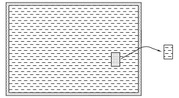
REMOVE FIBERGLASS OUTLINE ON EXTENSION WITH UTILITY KNIFE BEING CAREFUL NOT TO CUT FABRIC.
