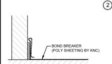
COVER FLOOR WITH BOND BREAKER (POLY SHEETING BY KNC), OVERLAPPING SEAMS A MINIMUM OF 6 INCHES, EXTEND UP OVER ISOLATION BOARD AND STAPLE TO WALL OR ROLL BACK ONTO FLOOR AND TAPE IN PLACE, ENSURE SEAMS ARE TAPED TO PREVENT CONCRETE FROM LEAKING THROUGH.
