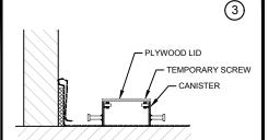
PLACE CANISTERS PER LAYOUT. CAULK OR TAPE CANISTER TO THE BOND BREAKER TO PREVENT CONCRETE FROM LEAKING BENEATH THE CANISTERS. INSTALL CANISTERS WITH PLYWOOD LID AS SHIPPED.
