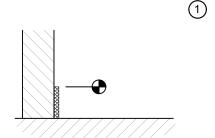
STRIKE FLOATING SLAB GRADE AND ADHERE RESILIENT INTERFACE (PPI BY KNC) TO PENETRATIONS AND PERIMETER LOCATIONS. SEE
